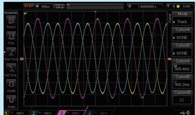
Three Phase Unbalance Voltage Test Captured
